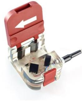
A high frequency voltage impulse is used to excite the piezo-ceramics and transmit ultrasound waves from one ceramic to the opposing one, with each one acting alternately as transmitter and receiver.
