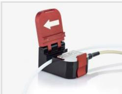
Too small tubing will create air spaces attenuating the signal.
