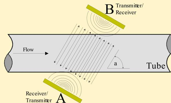
Figure 1: Principle of ultrasonic flow measurement (simplified using only two ceramics)
